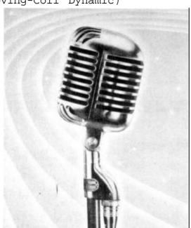
Low impedance models 55A and 55B may be fed into a standard low impedance input amplifier (See Fig. A-3) or into an amplifier with high impedance input (Fig. A-2). In the latter case Shure Model A86A Cable-Type Transformer is available for coupling the low impedance line to the amplifier input. The double-winding primary permits coupling either a 35-50 ohm line or 200-250 ohm line to the high impedance input.
