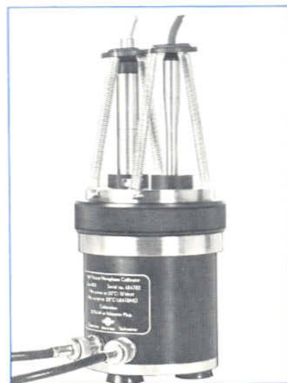
Fig.2. The High Pressure Calibrator set-up with two condenser microphones for comparison measurements
