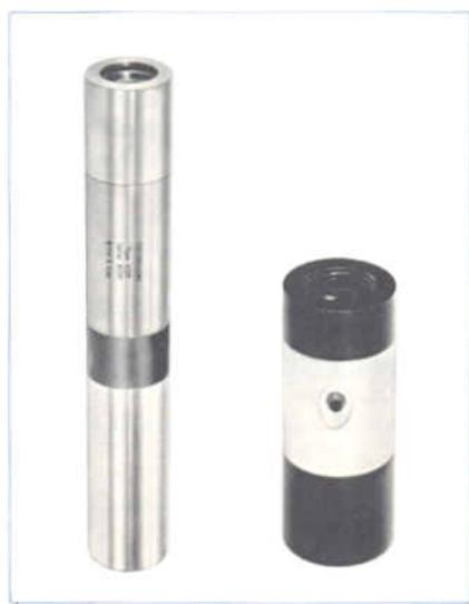
Fig. 17. Pistonphone Type 4220 and Sound Level Calibrator Type 4230
