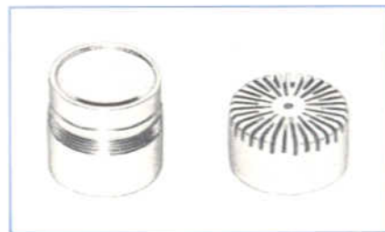
Fig. 3. 1" cartridge with protection grid removed. The diaphragm is flat and practically flush with the housing. This ensures a well defined acoustic impedance and excellent omnidirectivity
