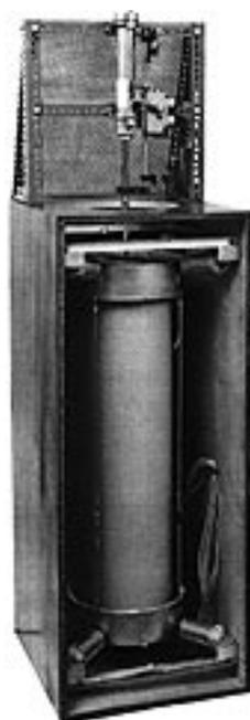
After 8 years of intensive study of mechanical reverberators (helical springs and other mechanical vibrating bodies), the BX20, the world's first, truly portable studio reverberator is ready for production. The spring reverb system design was practically finished and it took almost another year to design an appropriate suspension for it that would allow for safe shipping.
