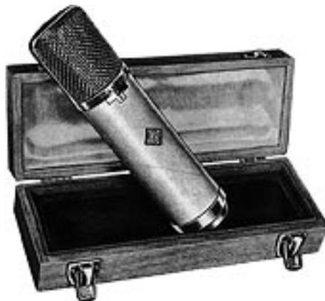
Rerun of the C 12 and several other versions for Telefunken and Siemens using the then advanced GE 6072 double triode.
